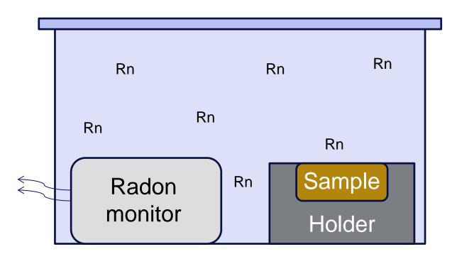
The most direct method uses a sensitive, constantly recording electronic monitor to give time-resolved radon measurements
