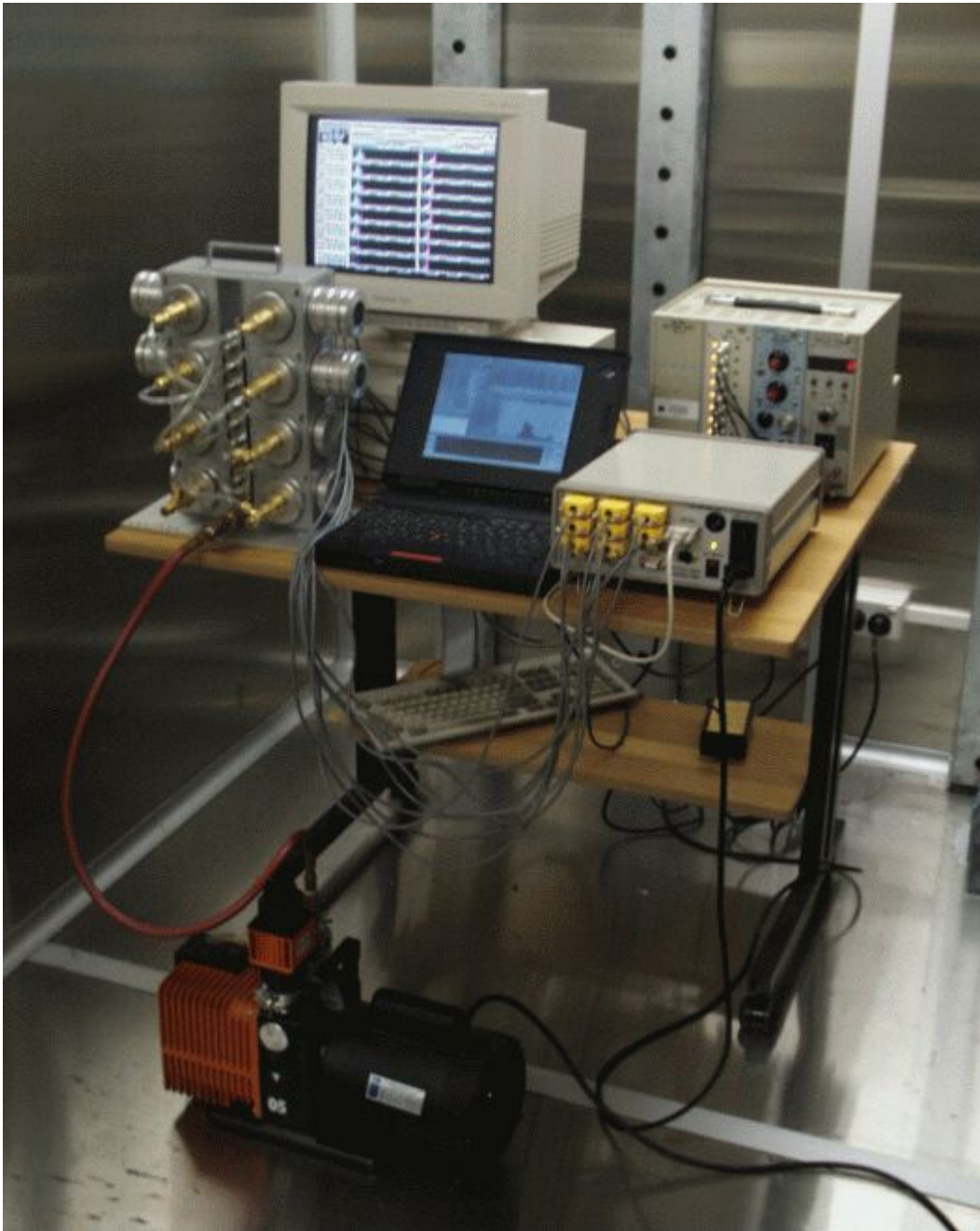
Fig. 1. Radon Progeny Particle Size Spectrometer (RPPSS)
