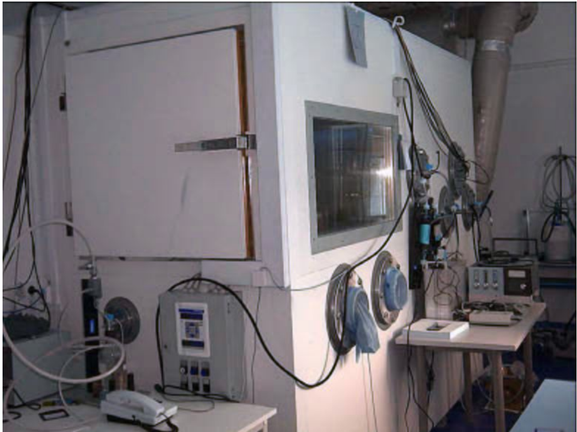
Fig.1. Radon chamber at CLOR
