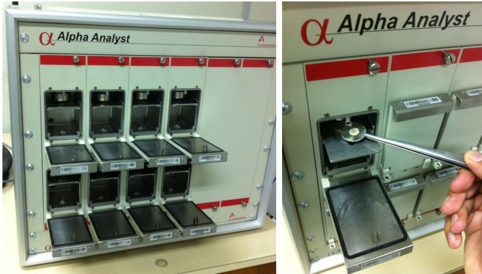
Measurement of Po-210 by alpha spectrometry during 80,000 seconds.
