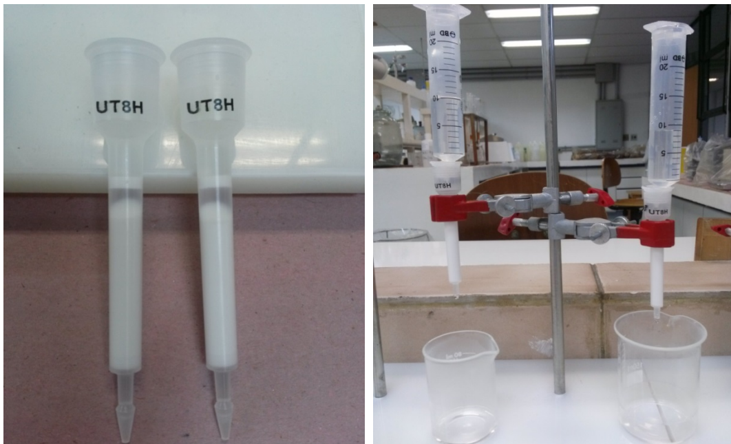
Examples of the UTEVA resin columns used for U and Th purification.
