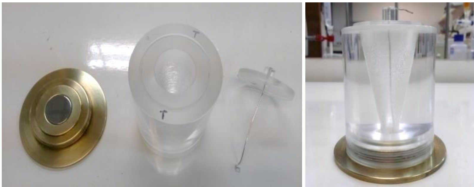
Example of the electrodeposition cell used in the experiment.
