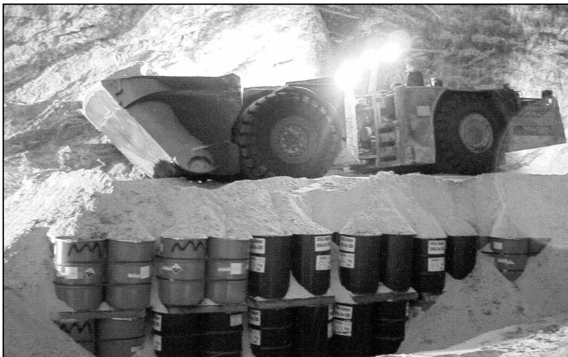
Fig. 4: Underground disposal in the salt cavern at Heilbronn.
