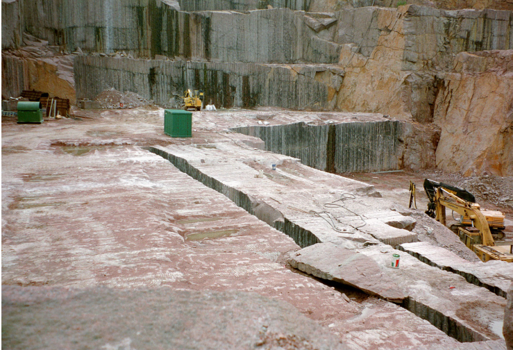
Figure 2. Extraction of granite blocks in the Vånga quarry.
