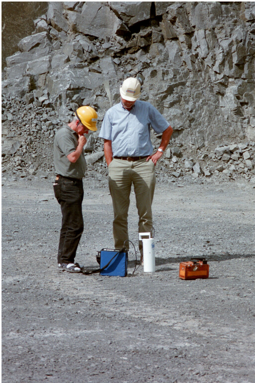
Figure 4. Gamma spectrometric measurement in the dolerite quarry.
