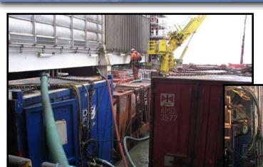
Slurrification of NORM through cuttings re-injection unit
