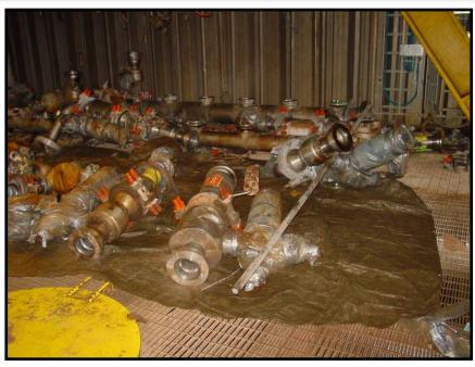
Cleaned process equipment (stainless steel) from Frøy.
