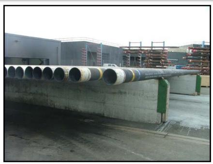
Cleaned production tubulars at Chemtech yard
