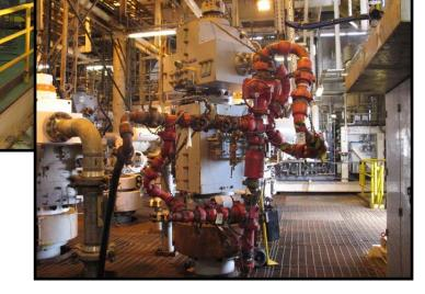
Injection of NORM slurry in waste well
