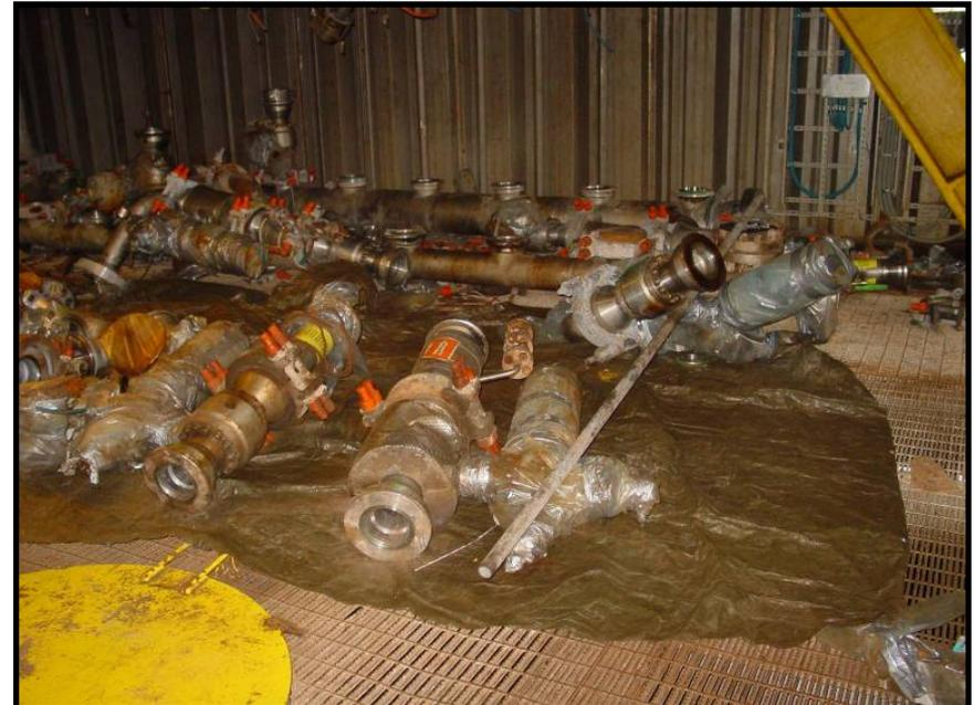
*Cleaned process equipment (stainless steel) from Frøy.*
