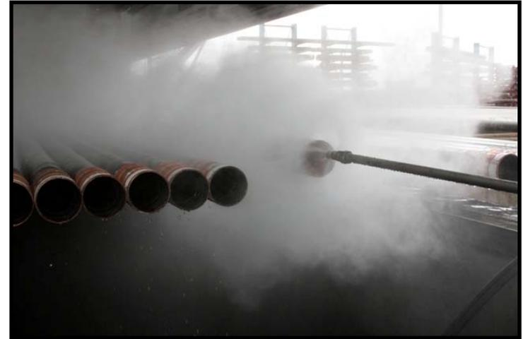
**HPWJ (> 2000 bar) has been the preferred NORM decontamination method in Norway since 1995. Several specially designed plants perform decontamination on a routine basis. The used water (with NORM) is collected in settling tanks before emission. The NORM material is retrieved and stored. The method works very well on easily accessible components, e.g. production tubulars. HPWJ does not create secondary waste, but releases activity to the environment (activity < 1 Bq Ra-226/litre)**
