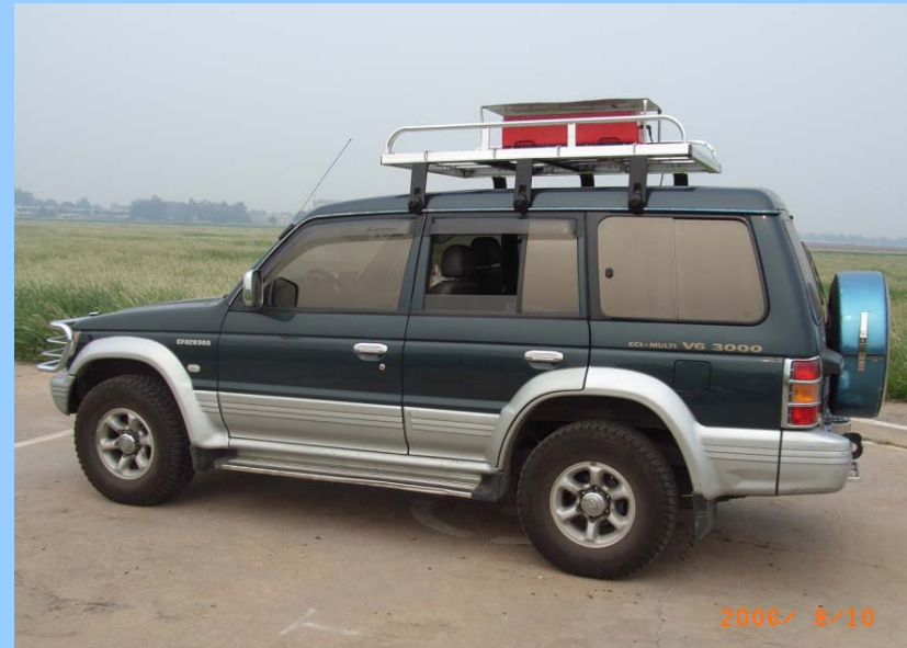
The CGS system was installed in jeep, with large volume(4L) , GR460 , NaI(Tl) detector.
