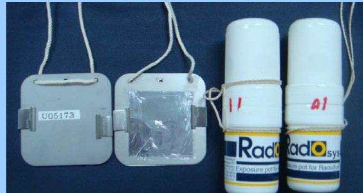
^{222}\text{Rn}/^{220}\text{Rn} and ^{220}\text{Rn} progeny CR-39 detector
