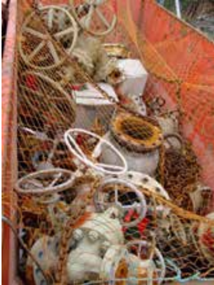
NORM contaminated valves
