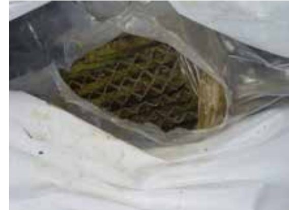
NORM contaminated plastic plates from separator
