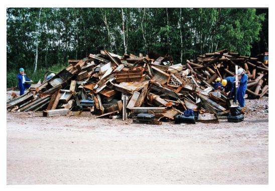
Randomly selected measuring points allows to determine parameters which are representative for the batch
