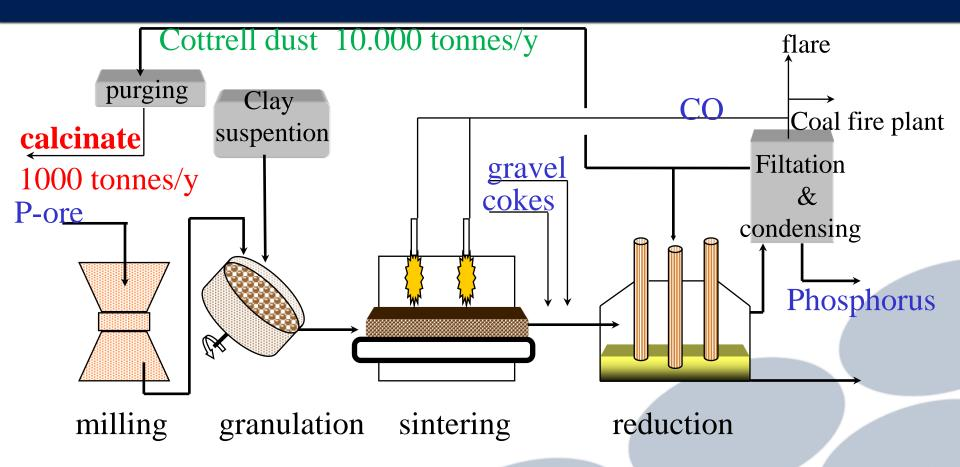
Phosphate ore + gravel + cokes => slag + Carbon monoxide+ Phosphor
