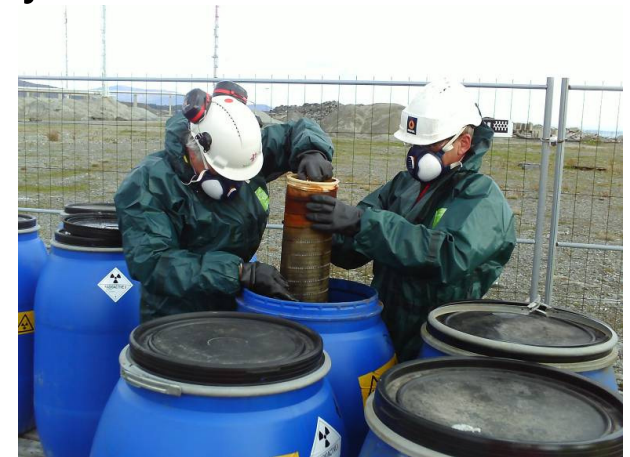
Filters with NORM from gas extraction. Radioactive and pyrophoric material
