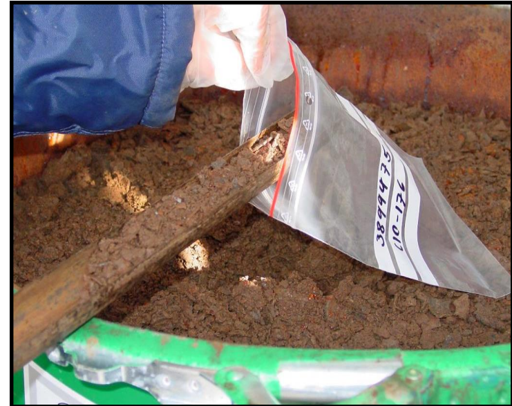
Sampling of LSA Scale containing sludge.
