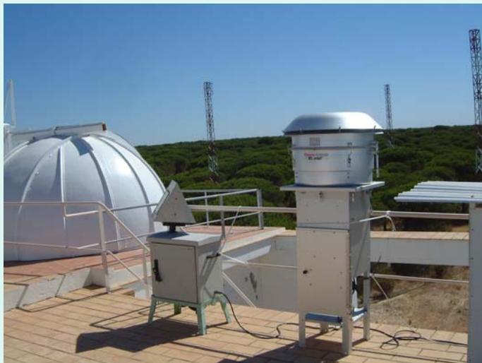
Aerosol collectors in background area
