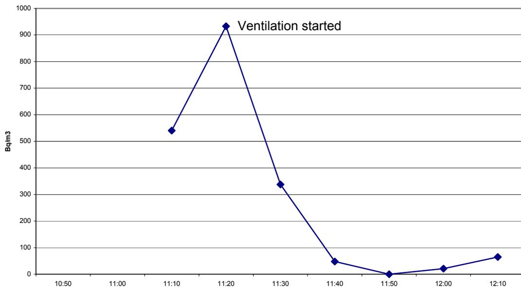
Fig.4: Radon measurements close to the mixing chamber at the Ludvika waterworks
