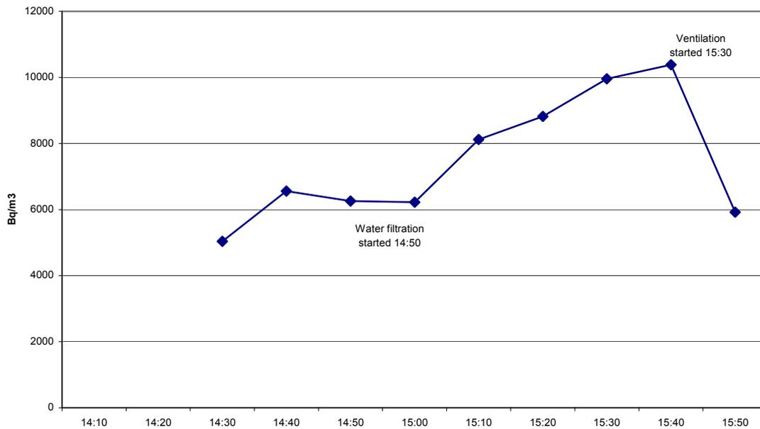
Fig.5: Radon measurements in the main hall at the Fredriksberg waterworks
