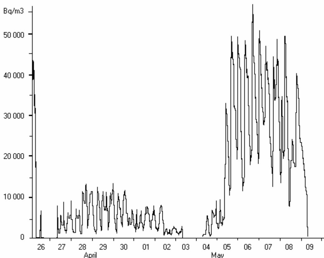
Fig.8: Radon gas measurements in the main hall at the Kolbäck waterworks
