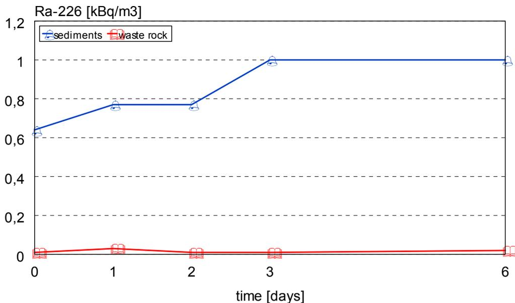
It can be seen, that the leaching of radium from waste rocks is negligible, especially in comparison with re-entry of radium into water from bottom sediments. We found in the filtrates from the experiments in which waste rocks were used, radium concentration at the levels close to values typical for groundwater in “normal” areas (below 0.1 kBq/m<sup>3</sup>). It means, that the increase of the radiation hazard due to the contamination of groundwater can be
