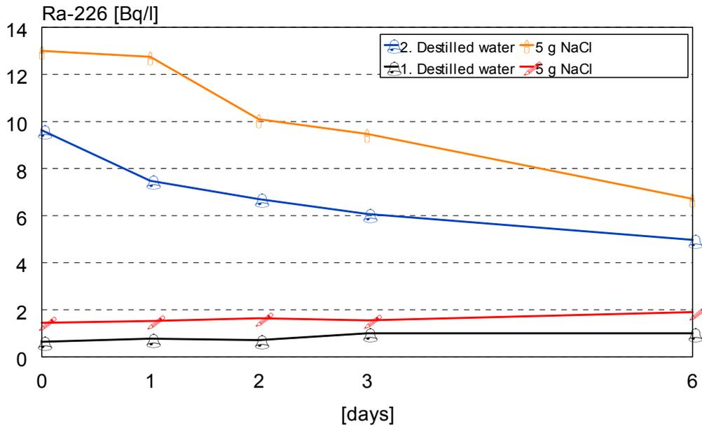
Fig.2. Comparison of the leachability of radium sample 1 from Bojszowy, sample 4 from Rontok
