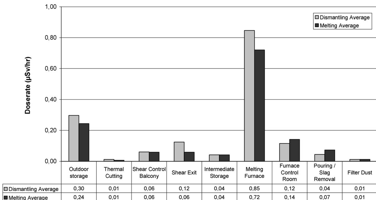
FIG. 3. Comparison of workplace dose measured by EPD for melting and dismantling
