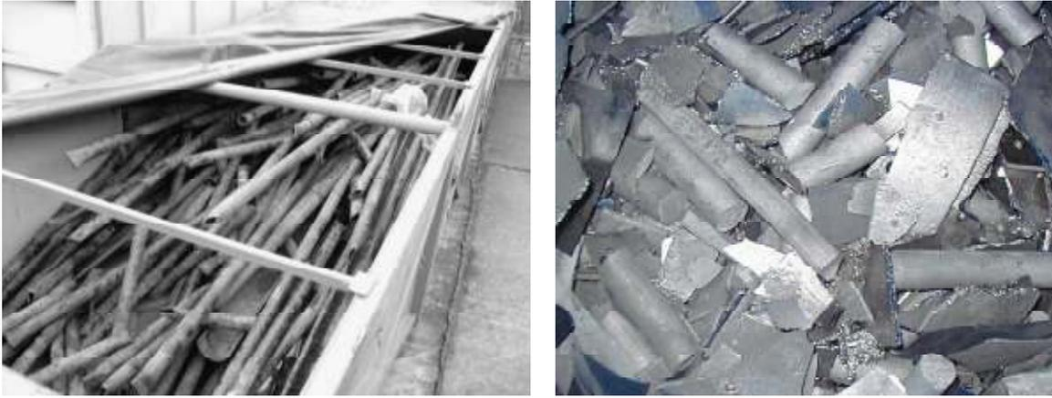
*FIG. 1. Example for contaminated pressure pipes from the oil and gas production industry and waste material from the tungsten welding production industry.*
