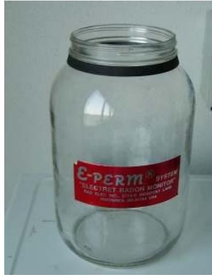
FIG.4. Electret ion chamber and glass jar of E-PERM<sup>®</sup> system
