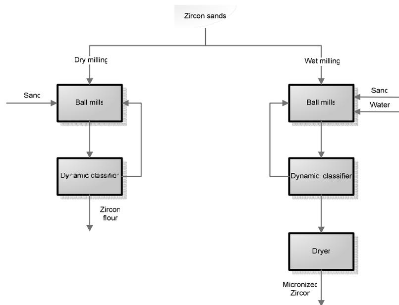
FIG. 2. Dry milling and wet milling processes
