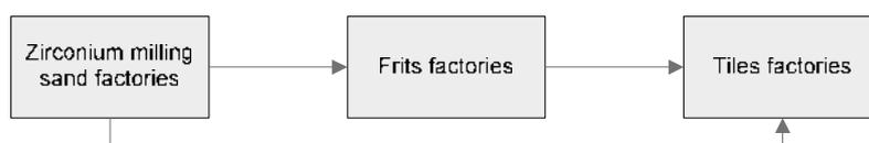
FIG. 1. Manufacturing processes using zircon sand
