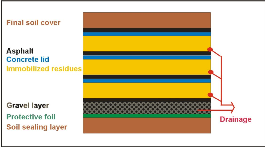
Fig. 2: Layered structure of the disposal facility for residues from the Aue WTP
