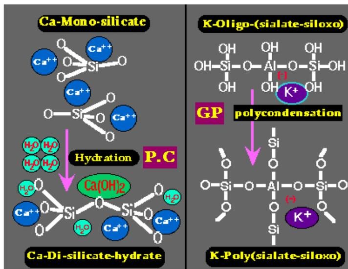
Figure 1: Comparison between Portland cement (P.C) and Geopolymer (GP)
