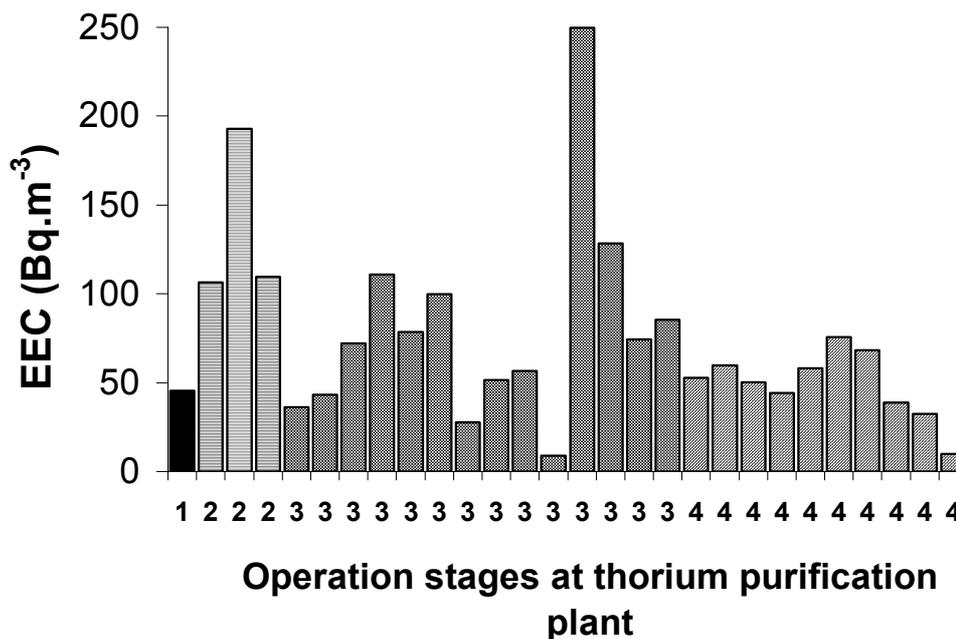
Figure 2: Thoron equilibrium equivalent concentrations (EEC) at stages of the thorium purification process between June/1997 and December/1998
